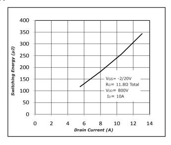
Fig 6. Inductive Switching Energy(Turn-on) vs ID
