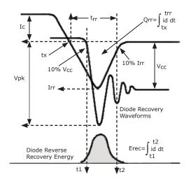
Fig 12. Body Diode Recovery Waveform
