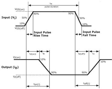
Fig 10. Switching Waveform Test Circuit
