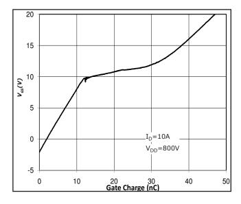
Fig 8. Typical Gate Charge Characteristics @ 25°C
