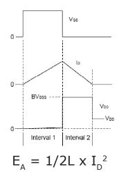
Fig 15. Theoretical Avalanche Waveform
