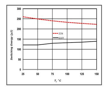
Fig 9. Inductive Switching Energy vs. Temp
