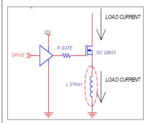
Kelvin gate connection with separate source return is highly recommended
