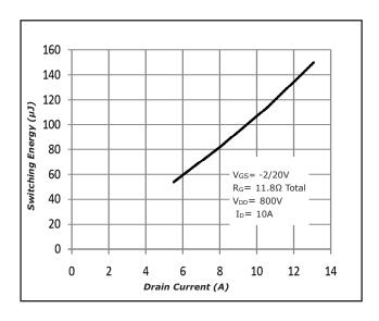
Fig 7. Inductive Switching Energy(Turn-off) vs ID
