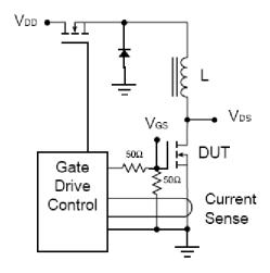
Fig 14. Avalanche Test Circuit
