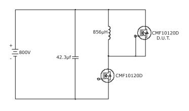
Fig 13. Body Diode Recovery Test
