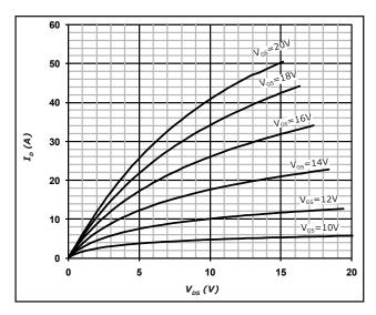
Fig 1. Typical Output Characteristics  $T_1 = 25^{\circ}C$
