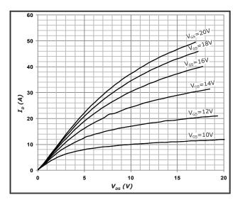
Fig 2. Typical Output Characteristics  $T_{\text{\tiny J}} = 150^{\circ}\text{C}$
