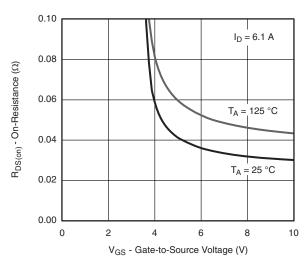
On-Resistance vs. Gate-to-Source Voltage
