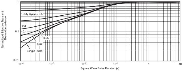
Normalized Thermal Transient Impedance, Junction-to-Foot
