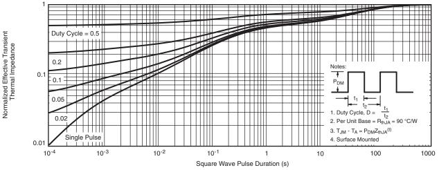
Normalized Thermal Transient Impedance, Junction-to-Ambient
