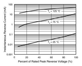
Fig. 4 - Typical Reverse Characteristics
