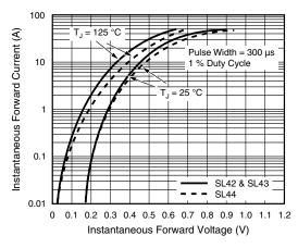
Fig. 3 - Typical Instantaneous Forward Characteristics
