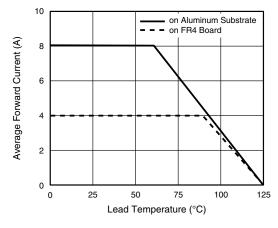
Fig. 1 - Forward Current Derating Curve
