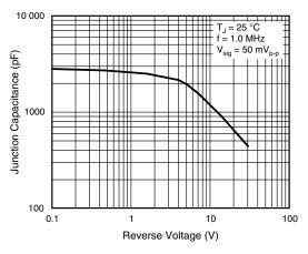
Fig. 5 - Typical Junction Capacitance
