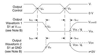
Voltage Waveform Enable and Disable Times
