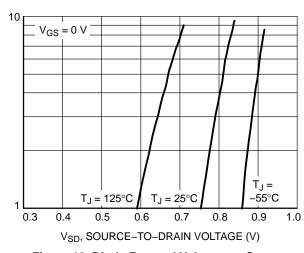
Figure 10. Diode Forward Voltage vs. Current
