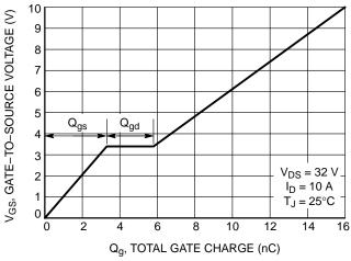
Figure 8. Gate-to-Source vs. Total Charge
