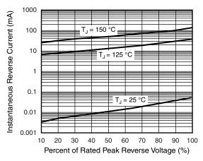
Fig. 4 - Typical Reverse Characteristics
