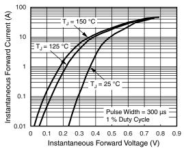
Fig. 3 - Typical Instantaneous Forward Characteristics
