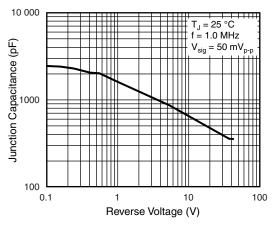
Fig. 5 - Typical Junction Capacitance
