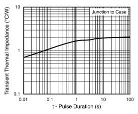
Fig. 6 - Typical Transient Thermal Impedance
