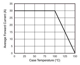
Fig. 1 - Forward Current Derating Curve
