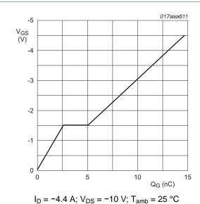
Fig 14. Gate-source voltage as a function of gate
