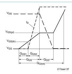
Fig 15. Gate charge waveform definitions
