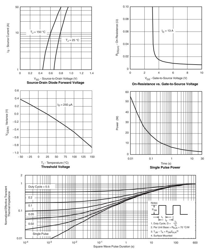
Normalized Thermal Transient Impedance, Junction-to-Ambient
