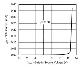
Gate Current vs. Gate-Source Voltage
