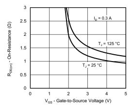
On-Resistance vs. Gate-to-Source Voltage
