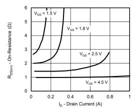
On-Resistance vs. Drain Current and Gate Voltage
