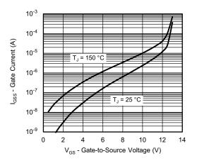
Gate Current vs. Gate-Source Voltage
