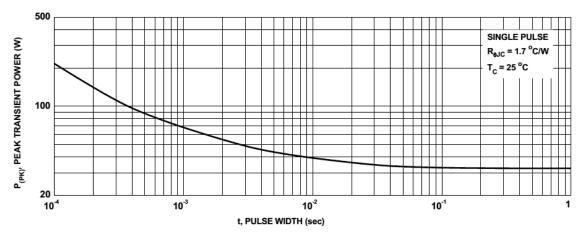
Figure 13. Single Pulse Maximum Power Dissipation
