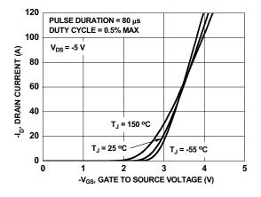
Figure 5. Transfer Characteristics
