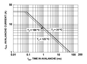
Figure 9. Unclamped Inductive Switching Capability
