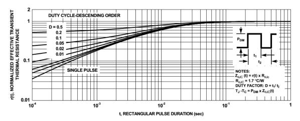
Figure 14. Junction-to-Case Transient Thermal Response Curve
