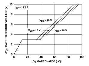
Figure 7. Gate Charge Characteristics
